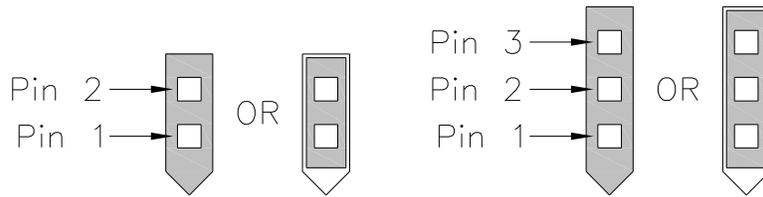
**Figure 3.2: Jumper-pin numbering for 2- and 3-pin jumpers**
