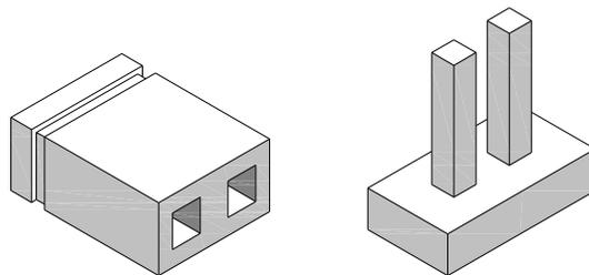
**Figure 3.1: Jumper block and pins**
